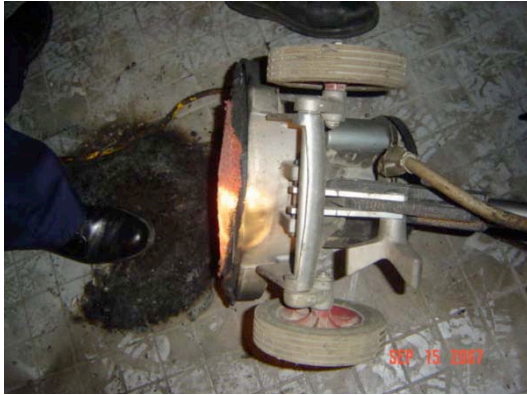
This electric scrubber, used in cleaning the floor with the organic solvent, was a key suspect as the source of ignition.
